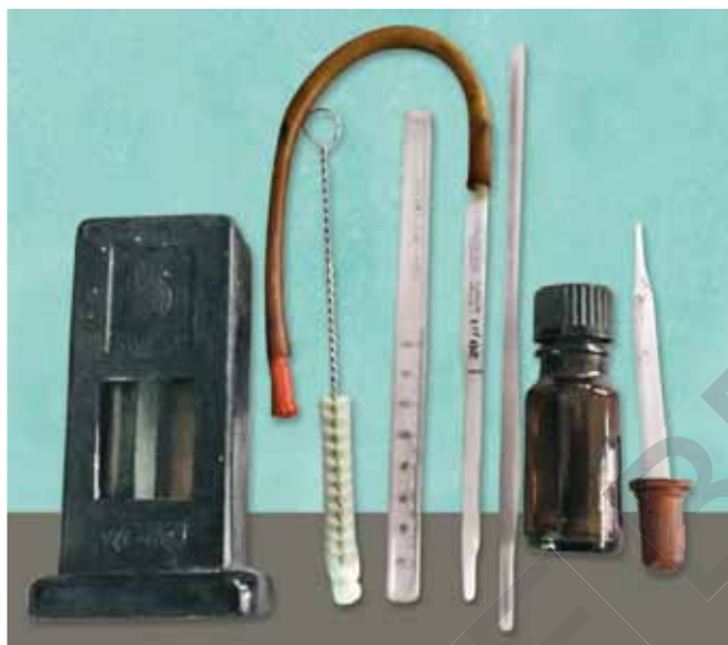
Fig. 6.1: Sahli's hemoglobinometer showing the box with standard color, brush, diluting tube, pipette, glass rod, N/10 HCl and dropper.
