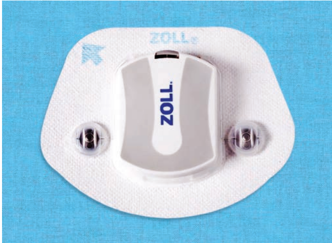
FIG. 6: \mu Cor wear-on patch (Zoll) patch for detection of abnormal heart rhythms.
