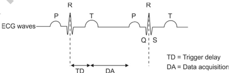
**FIG. 1:** Diagram of ECG gating.
