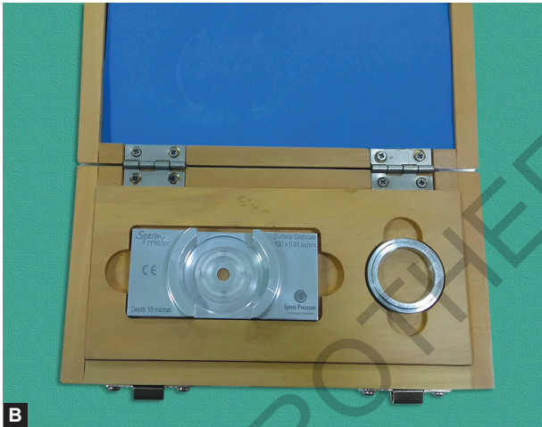
Figs. 4.3A and B: Indian cryo cell sperm counting chamber.
