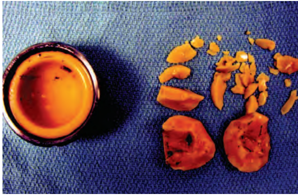
Figure 8: Photograph depicting ceramic head fracture. From D'Antonio JA, Sutton K. Ceramic materials as bearing surfaces for total hip arthroplasty. J Am Acad Orthop Surg. 2009;17:63-8, with permission.
