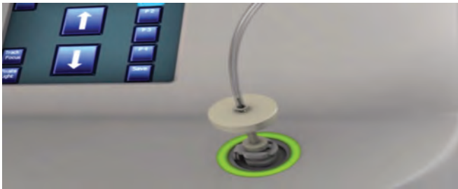
Fig. 7 Connection of the suction tube
