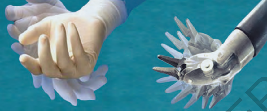
Figure 1.8: Seven degrees of movement (Endowrist technology)
