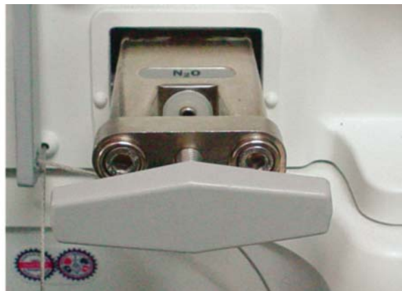
Fig. 4.7: The hanger yoke assembly: shows retaining screw opened (l) and in place (r). note bodok washer and pins
